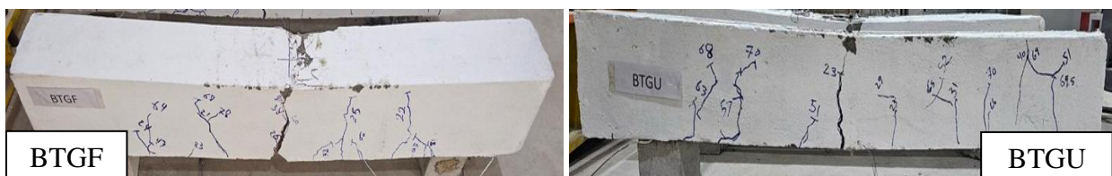
C. Failure Mode and Crack Pattern of Group 2.
