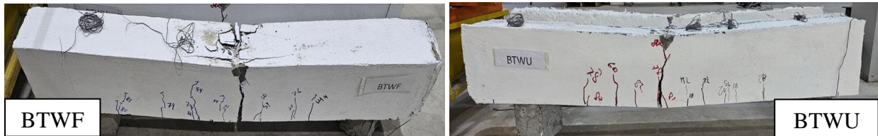
B. Failure Mode and Crack Pattern of Group 1.
