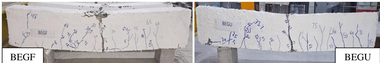
E. Failure Mode and Crack Pattern of Group 4.
