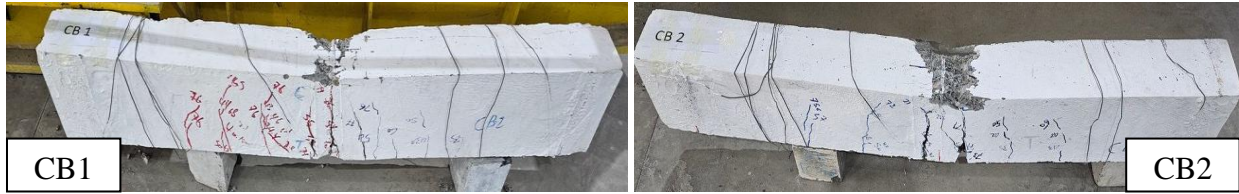
A. Failure Mode and Crack Pattern of Control Beams.
