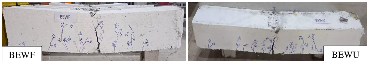
D. Failure Mode and Crack Pattern of Group 3.
