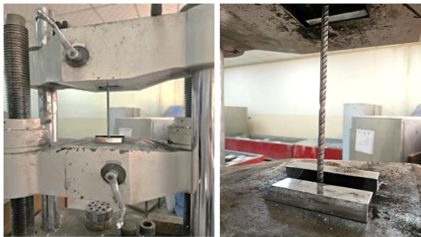
Figure (3.6): Steel Reinforcement Specimens and Testing Machine
